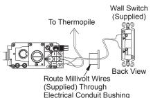
Figure 11 - Wall Switch Installation
